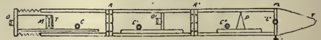
O, O', lenses; M, single lenses; T, screen; C, C', C'', rack and pinions; R, R', hinges; P, prism; Pl, plate; L, L', micrometric screws; V, eye-hole.
